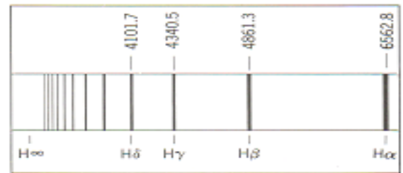
Fig. 6. A schematic spectrogram for the first few spectral lines of the Balmer Series.
