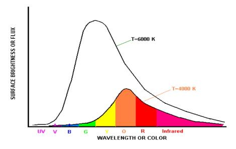
The above diagram depicts a plot of Planck's Law for two different temperatures. It shows how the brightness varies with wavelength over the spectrum for an incandescent body, such as stars.
