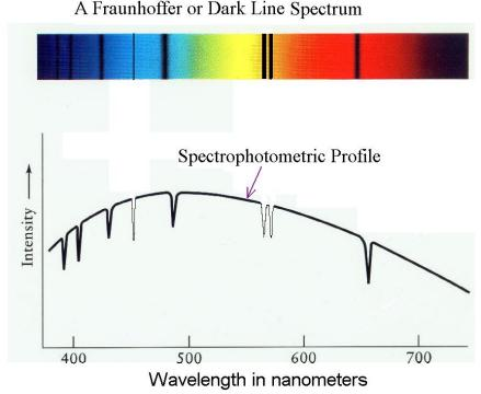
Most stars exhibit a dark line or absorption spectrum. That is, a continuous spectrum with discrete wavelengths weakened by atoms absorbing radiation at these wavelengths. Such a spectrum is also called a Fraunhoffer spectrum. An example is shown in the diagram above.
