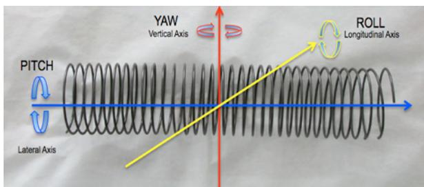
Figure 3. Spring's three axes of rotation
