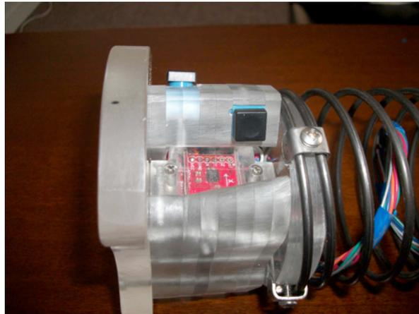
Figure 4. Accelerometer and two of the five buttons
