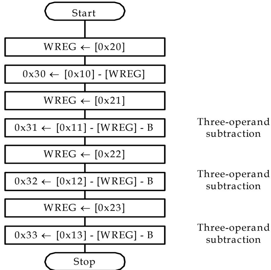
Figure 2.2 Logic flow of Example 2.7
