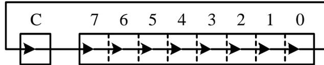
Figure 2.19 Operation performed by the **rrcf f,d,a** instruction
