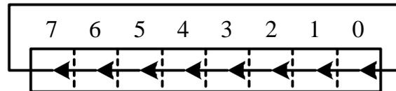
Figure 2.18 Operation performed by the **rlncf f,d,a** instruction
