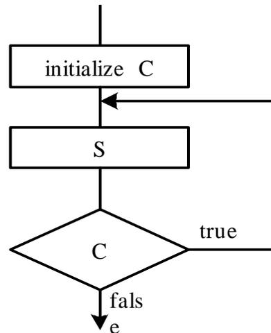
Figure 2.8 The **Repeat ... Until** looping construct
