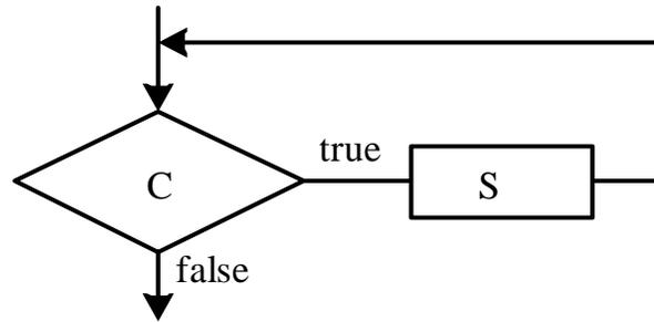
Figure 2.7 The **While ... Do** looping construct
