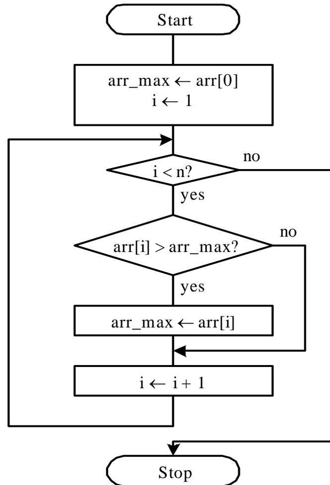
Figure 2.13 Flowchart for finding the maximum array element
