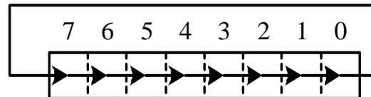
Figure 2.20 Operation performed by the **rrncf f,d,a** instruction
