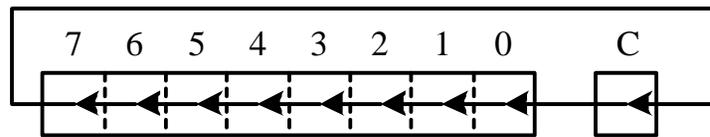
Figure 2.17 Operation performed by the **rlcf f,d,a** instruction
