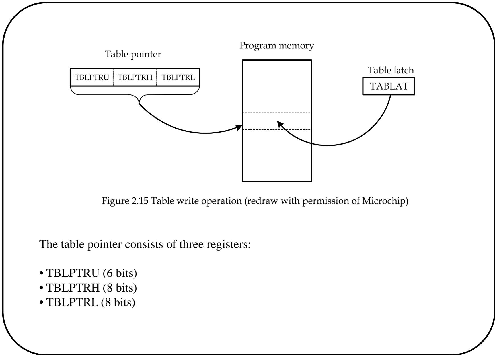
Figure 2.15 Table write operation (redraw with permission of Microchip)
