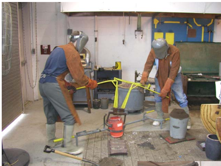
Molten aluminum was removed from the furnace in preparation for pouring.
