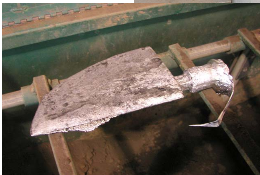
The rough casting was then broken out of the mold in preparation for the finishing processes.
