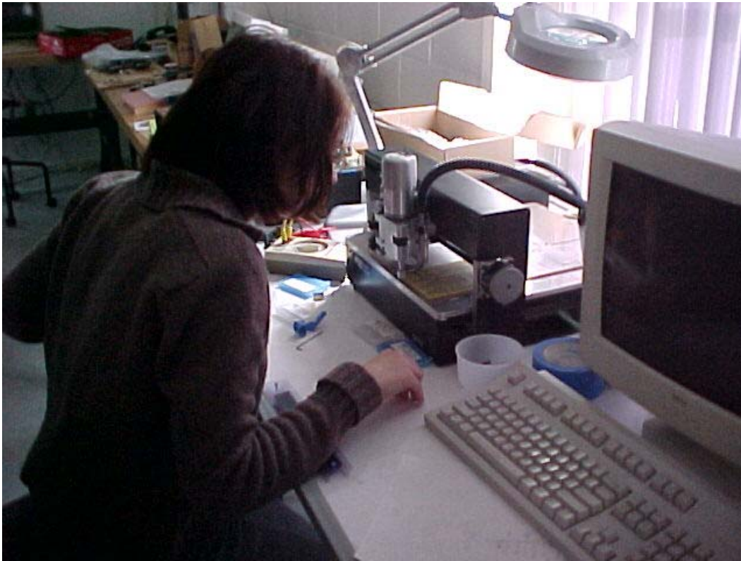
Above, Marian is machining one of the several circuit boards for the two controllers. The proof is in the testing. Below, Marian presses on the foot pedal switching the solenoids through the three different voltages.
