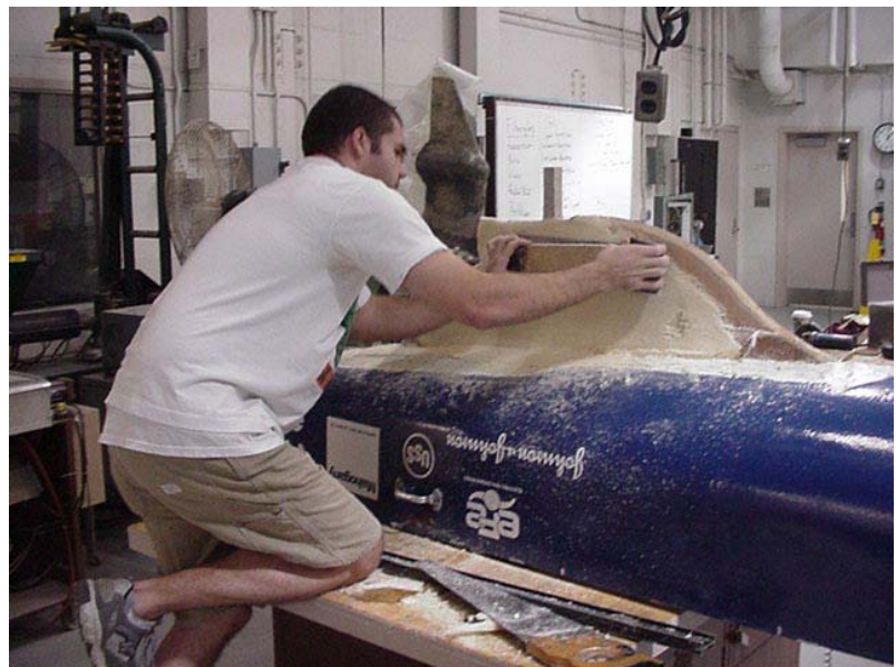
Joe shaping foam keel in preparation for fiberglass.
