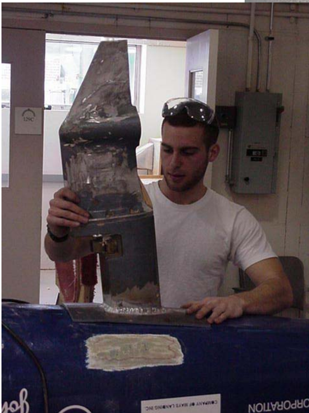
Fitting entire drive unit to bottom of hull.
