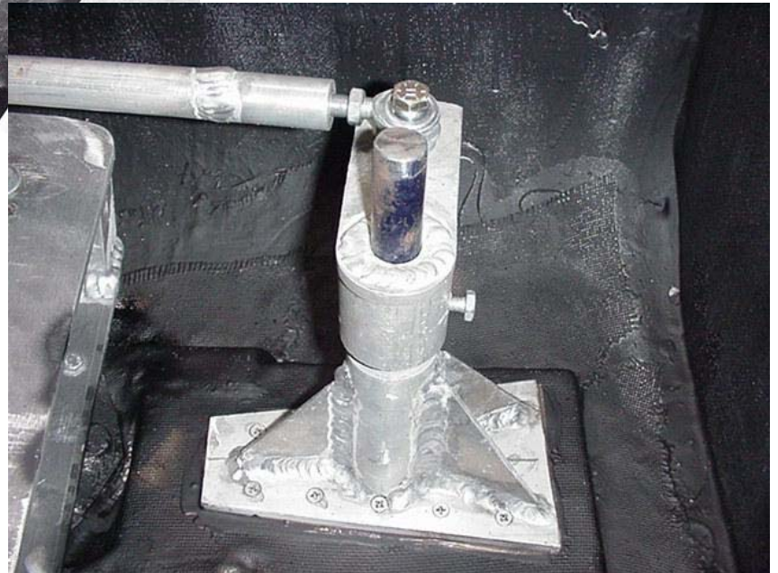
Tiller assembly. Actuated by "teleflex" cable and steering wheel.
