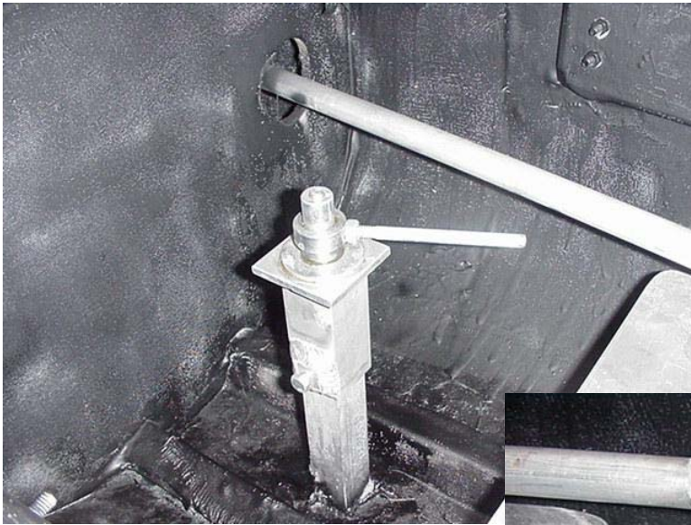
Rear wing adjuster. Can change angle of attack of rear wing between sprint wings and endurance wings. Angle can also be changed between drivers. Tiller rod in background.
