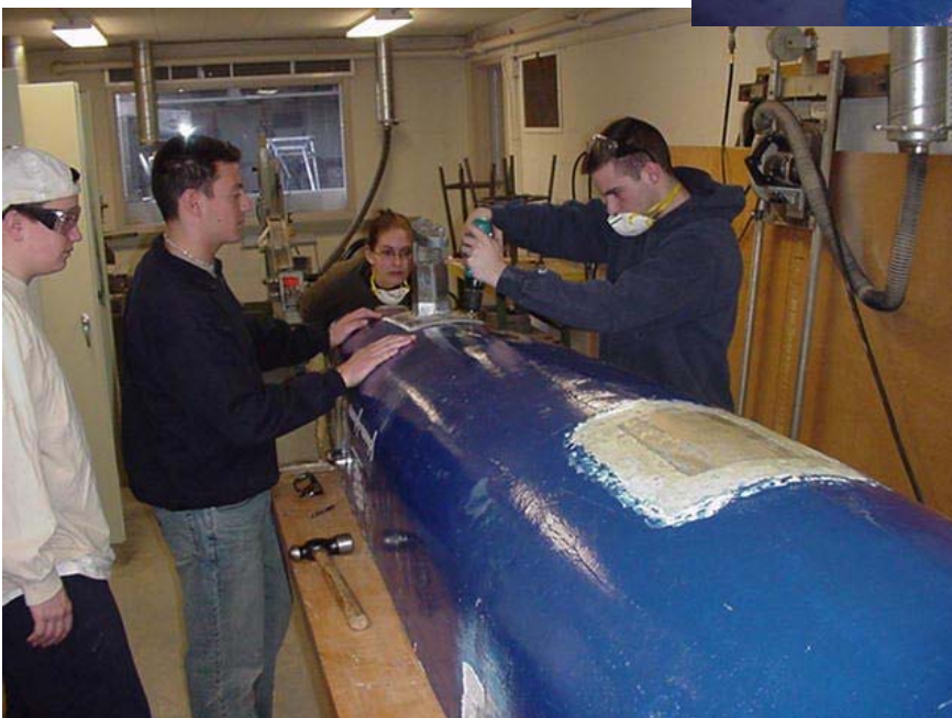
Screwing lower unit and fiberglass sandwich to bottom of hull. Patch in foreground fills the drive unit opening used in the 2000 boat.
