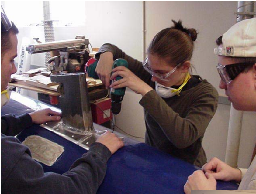
Marian drilling mounting holes to attach lower unit.
