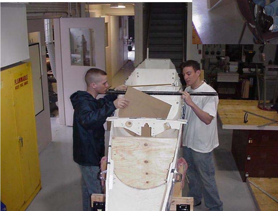
Locating seat back, helm, and hydrofoil support bulkheads.
