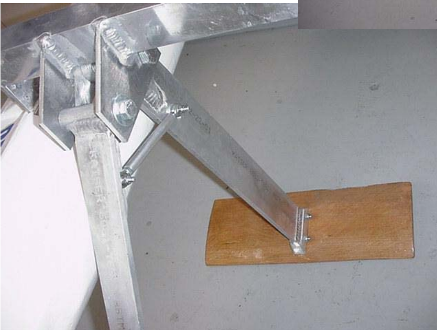
Connecting/adjusting link between skimmer arm and wing supporting column.
