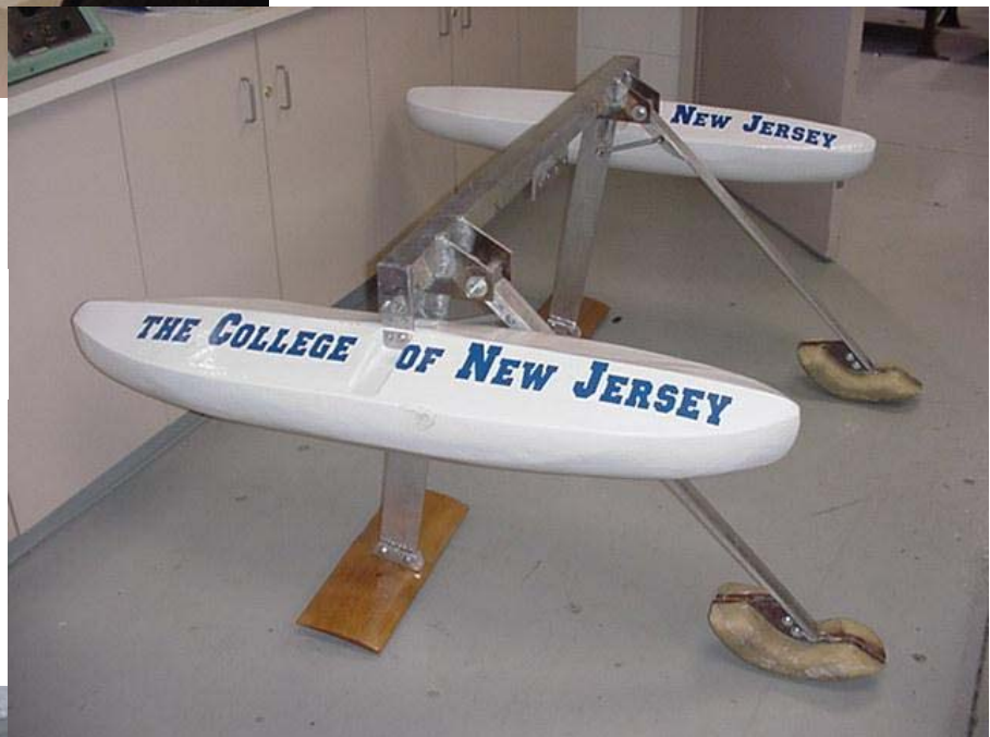
Connecting/adjusting link between skimmer arm and wing supporting column.
