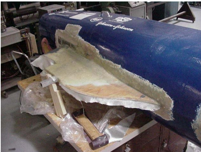
Fiberglass applied to foam and plywood keel.
