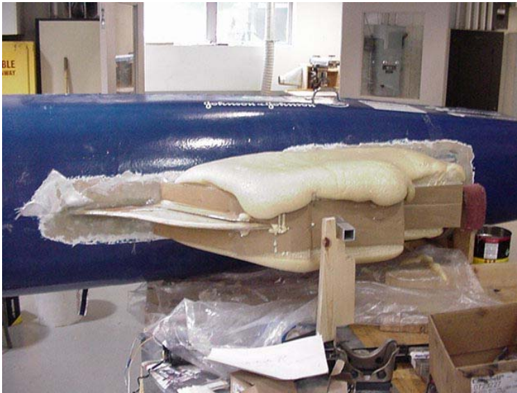
Casting A-B foam to shape keel/drive unit support. Aluminum post in center is mount for main hydrofoil.
