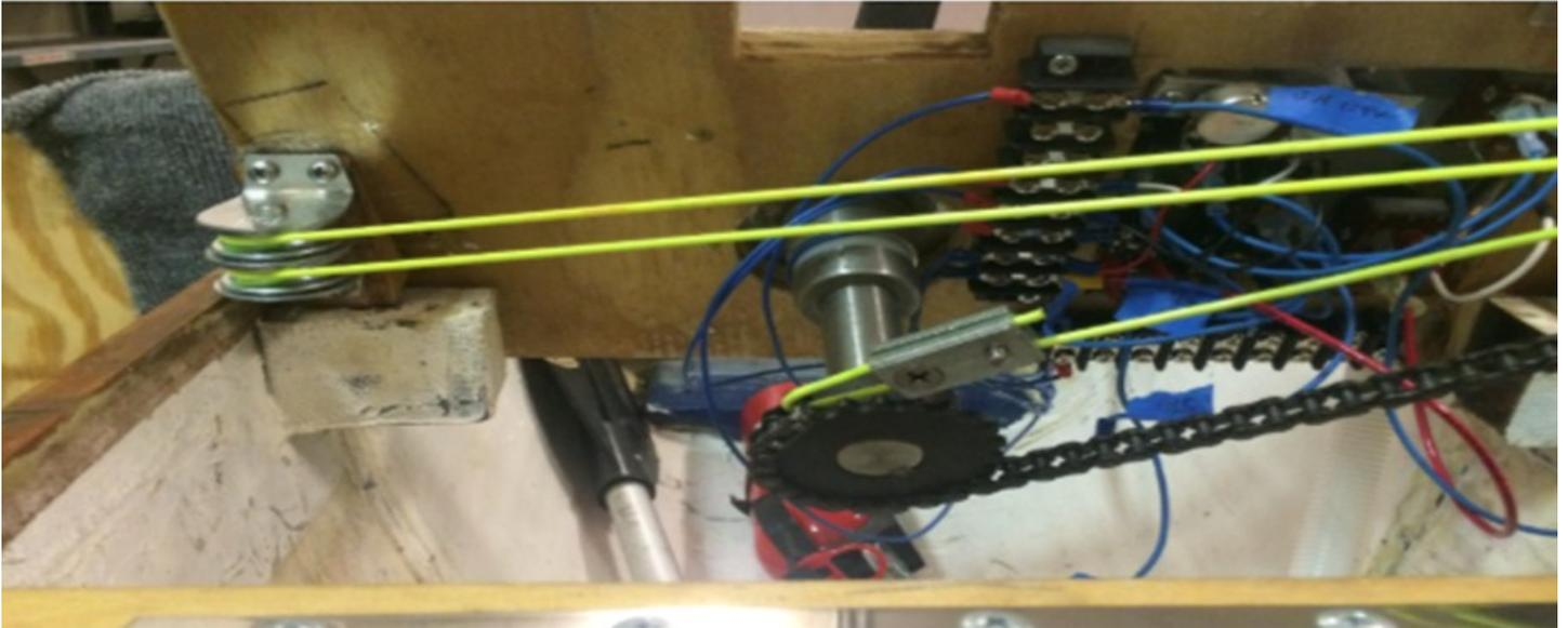
The Helm consists of a standard sprocket mounted to the wheel shaft. The chain and sprocket mechanism then drives a standard cable/tiller steering system.
