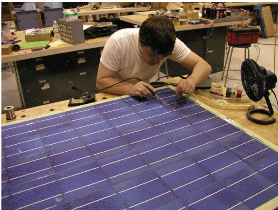
Brad endures the tedium of soldering the solar cells into an array. It's a relief to finally solder the cells to a bus bar.
