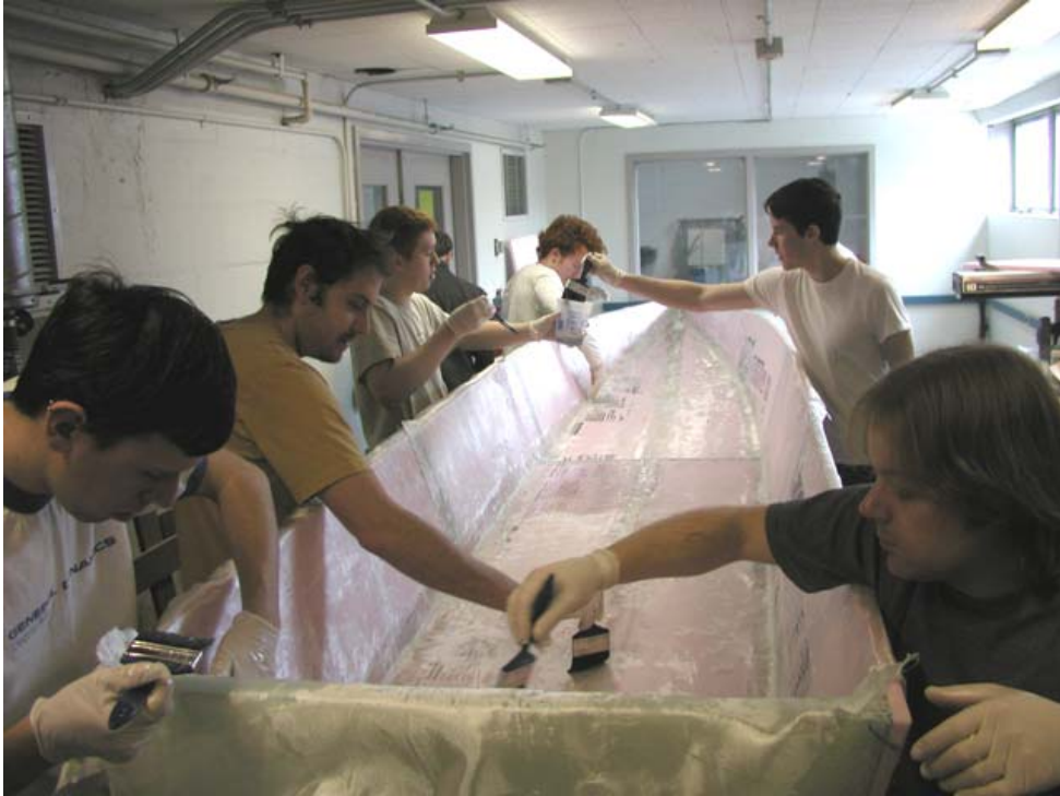
The fiberglass applied to the inside of the hull was hand laid. Again, many hands make for quick work.
